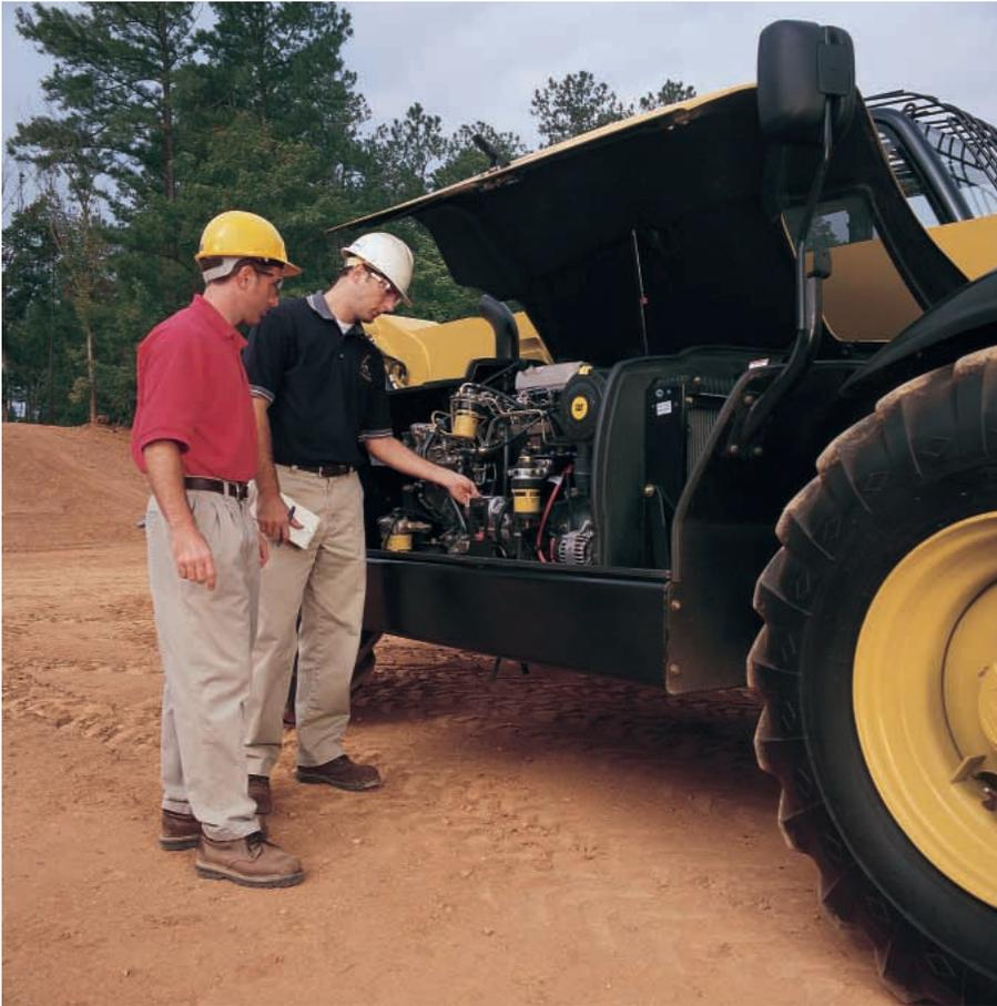
**Access.** All Cat Telehandler service points, including the combined transmission/hydraulic oil filter, are readily accessible and major components are easy to reach at ground level due to the overall machine design.
