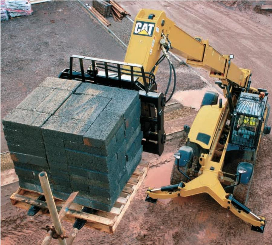
**Quick Coupler.** An IT interface is standard on the B-Series.
