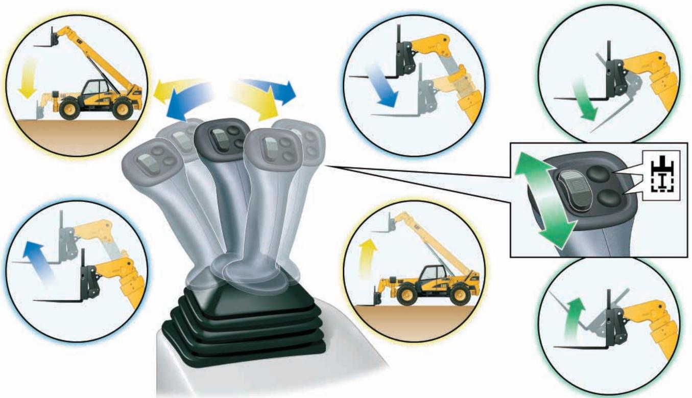
**Joystick Control.** The joystick allows three simultaneous boom functions and incorporates a unique slider switch.
