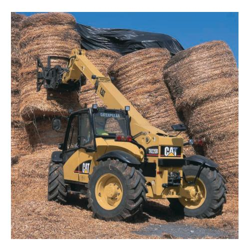
**Quick Coupler.** An IT interface is standard on the B-Series. For optimum versatility, all machines are equipped with the hydraulic quick coupler, allowing the operator to quickly and easily change non-hydraulic work tools without leaving the cab.
