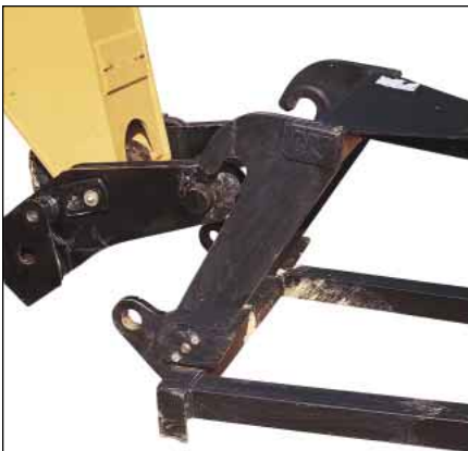
Line up quick coupler with tool
