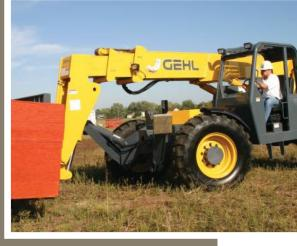
The RS Series Telescopic Handlers perform brilliantly on tight jobsites due to their tight turning radii and low overall height. The RS5-19 has a turning radius of 11'. The tight turning radius on the RS Series requires less backing up, which increases productivity and efficiency.
