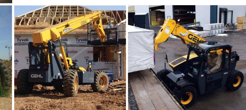
NEW Model RS5-19 **Size does matter . . . especially when working on confined jobsites.** Standing 6'4" with a turning radius of only 11', this little giant makes working in confined spaces easy. With a lift height up to 19'1" and a maximum load capacity of 5,500 lbs., the RS5-19 Telescopic Handler creates big results, maximizing your investment.
